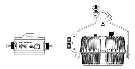
1 Connect OUTPUT port and W2K unit using RJ45 cable.
